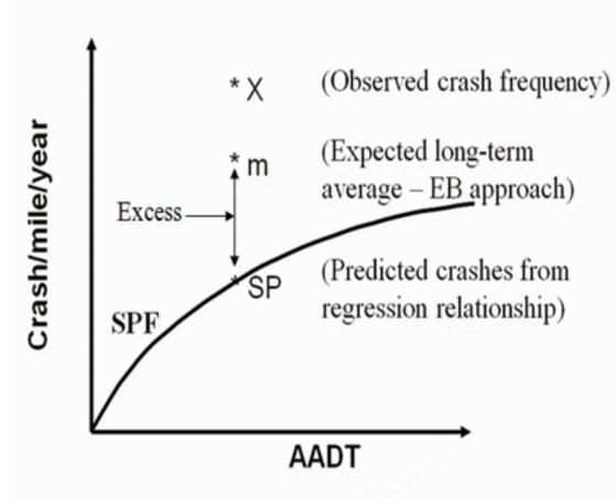
models to roadways with similar site types, i.e. 3-legged rural intersections with a minor stop control are modeled separately from 4-legged signalized urban sites. While the initial output of the model is predicted average crashes, the **Empirical Bayes** method can be applied to derive both expected average crashes as well as **Excess Expected Crashes (EEC)**, the difference between expected and predicted crashes.
